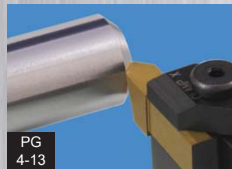
INTERNAL AND EXTERNAL CHAMFERING 45°
