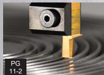
FOR TREPPANNING ON A CNC OR CONVENTIONAL MILLING MACHINE
