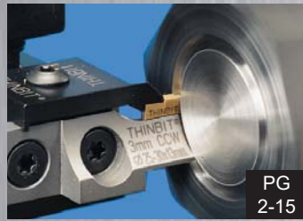
MAJOR DIAMETERS FROM .787"; 1" D.O.C.; 2, 3, 4, 5 AND 6MM INSERT WIDTHS
