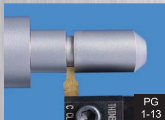
STATIC O-RING GROOVING WITH 1.250" MINIMUM BORE DIAMETER
