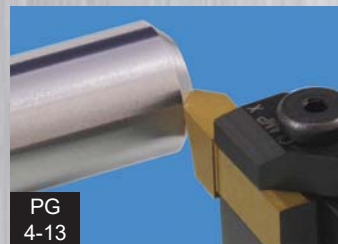
INTERNAL AND EXTERNAL CHAMFERING 45°
