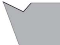
TOP RAKE (SIDE VIEW)
